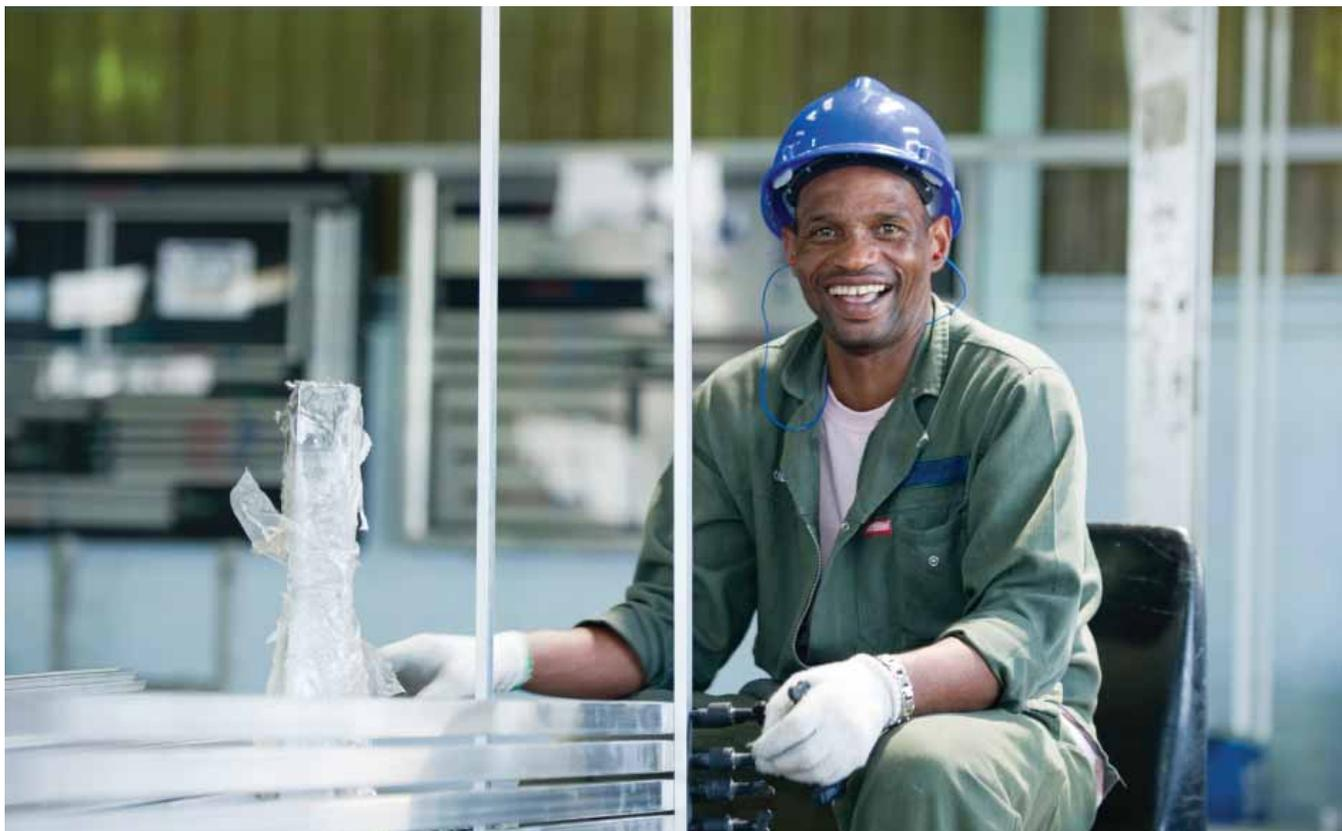
VK "Kido" Daniso, jiggling aluminium extrusions onto a flight bar in preparation for anodising
